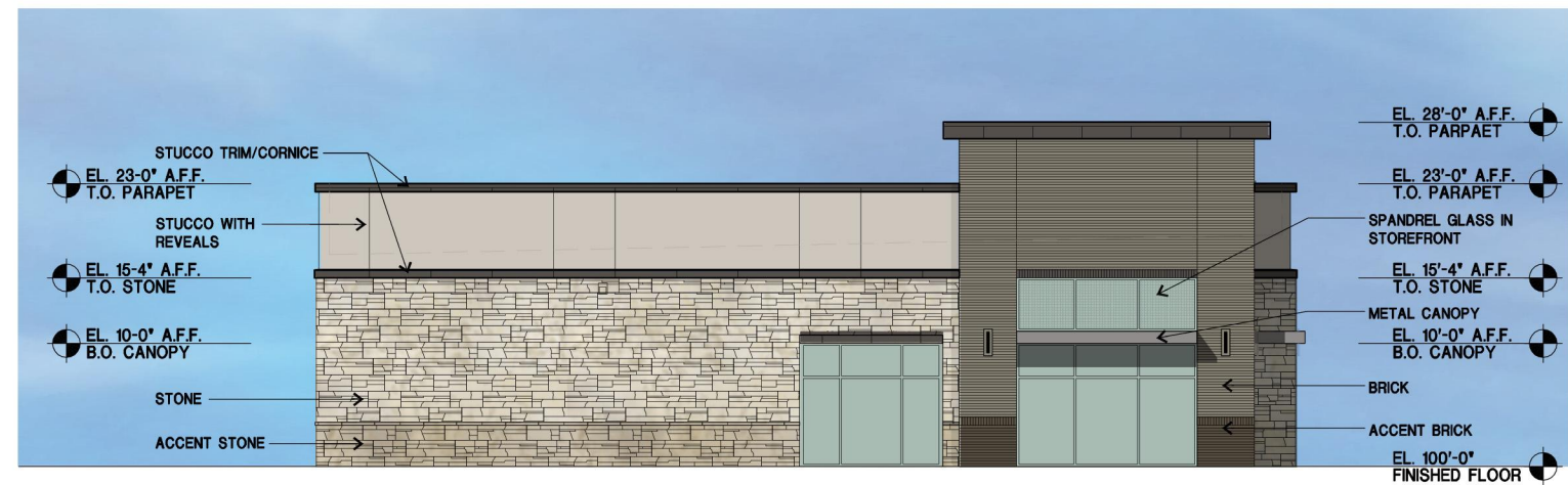
04 NORTH ELEVATION SIDE 1/16"=1'-0"
