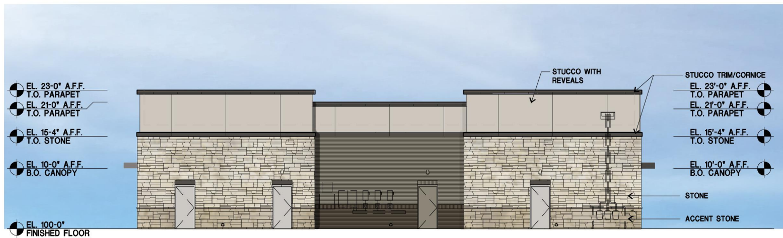
03 EAST ELEVATION REAR 1/16"=1'-0"
