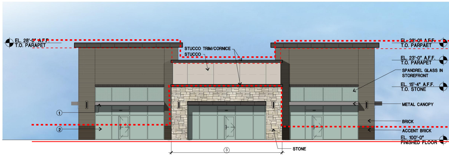
01 WEST ELEVATION FRONT 1/16"=1'-0"
