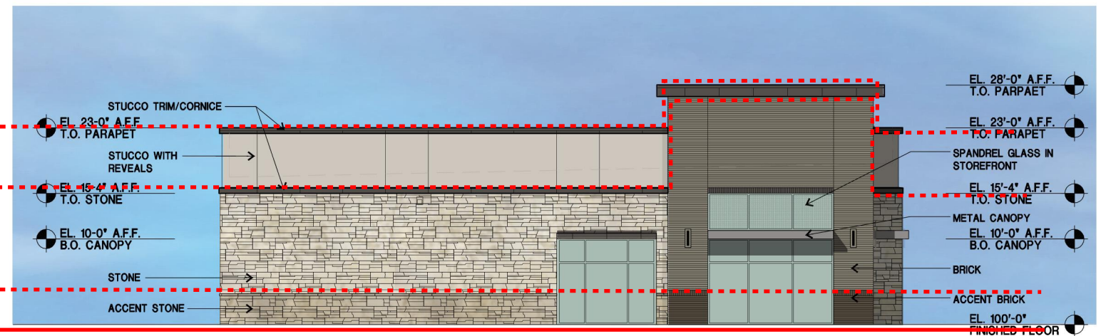
04 NORTH ELEVATION SIDE 1/16"=1'-0"
